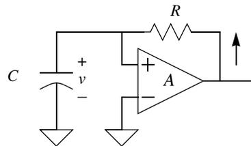
This model is used to develop a formula that gives the output voltage at the time it will be sampled versus the input voltage. In this circuit
