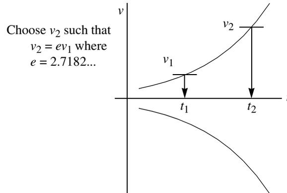
Pick an arbitrary voltage  $v_1$  at  $t_1$  and then measure the time it takes for the voltage to reach the voltage  $v_2$  where  $v_2 = ev_1$  with both measured with respect to the 0 crossover state (common mode of comparator output). Now
