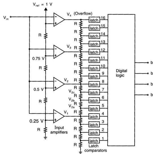
Define  $Q$  to be the quanta size at the input to the converter, as illustrated in Figure 4. So  $Q$  is the maximum amount of change in the voltage at the input that can be made without causing a transition in the output of an ADC. Including the effect of an input amplifier, the size of quanta at the latch input is  $QA_{UL}$ .
