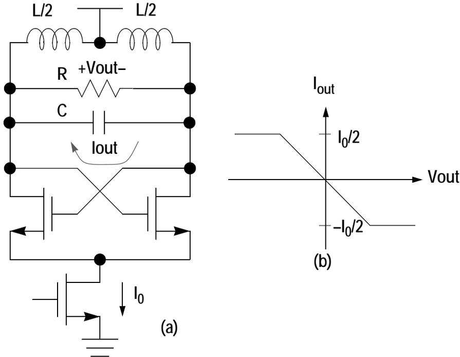
into the differential tank resistance is thus switching between  $I_0/2$  and  $-I_0/2$ . Some references use a different notation where the output current is taken as the difference between the currents in each side of the oscillator. In that case, the switching waveform moves between  $-I_0$  and  $I_0$  but flows into  $R/2$  to build the amplitude.
