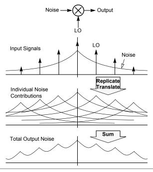
Noise from the source at a particular frequency f is replicated and copies appear at  $f \pm kf_0$ , where k is an integer and  $f_0$  is the fundamental frequency of the periodic signal. Conversely, noise at the output at a particular frequency f has contributions from noise from the sources at frequencies  $f \pm kf_0$ .
