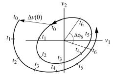
Consider plotting two state variables for an oscillator against each other, as shown in Figure 7. In steady state, the trajectory is a stable limit cycle, v. Now consider perturbing the oscillator with an impulse and assume that the response to the perturbation is  $\Delta v$ . Separate  $\Delta v$  into amplitude and phase variations,
