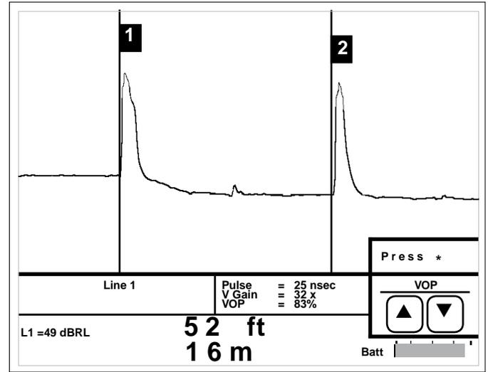
Mechanical inner-connectors (known as bullets) connecting sections of broadcast transmission line sometimes burn open causing power outages. These bullets can be detected by a TDR.
