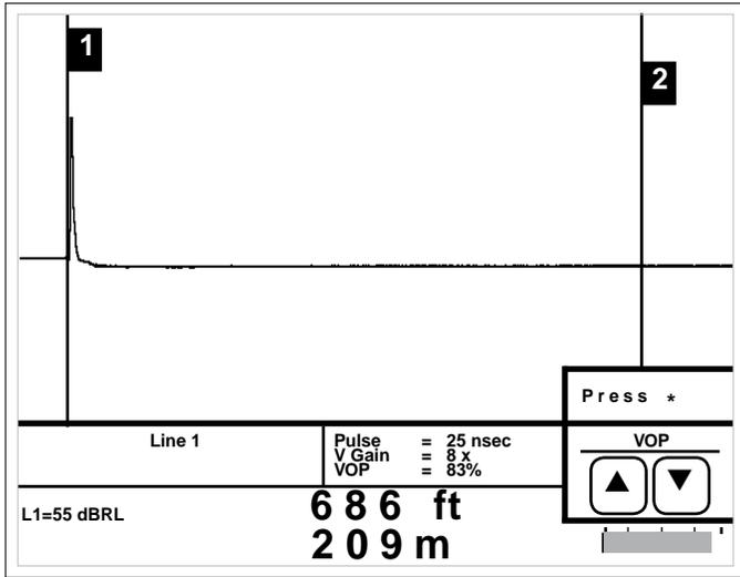
A properly TERMINATED cable will absorb the TDR signal, resulting in no reflection. Faults prior to the termination may appear as reflections along the waveform.
