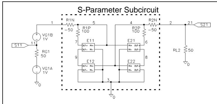
**Figure 21** *S-parameter subcircuit schematic also showing setup for evaluating  $S_{11}$  and  $S_{21}$ .  $Z_0=50$  ohms is assumed.*
