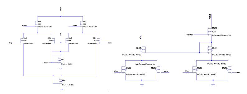
These topologies deteriorate the output swing as they are sensitive to the differential outputs as well
