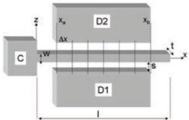
Schematic shows beam resonator slices into  $N$  sections using method of difference ( $N = 6$ ) in this case between  $x_a$  and  $x_b$
