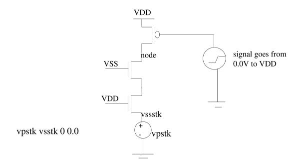
.measure tran avgleakagestk AVG i(vpstk) FROM='ckper+(cktr/2)' TO='ckper+(cktr/2)+(ckper/2)'
