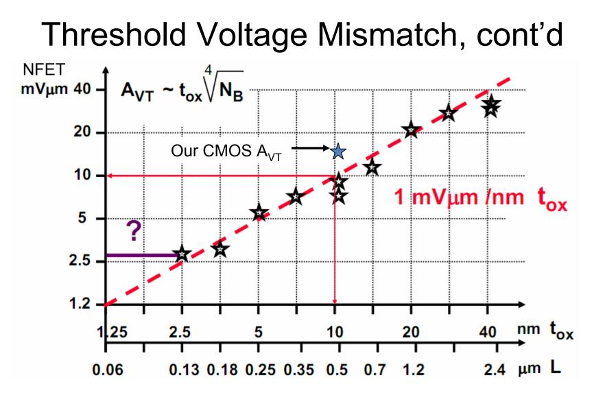
From W. Sansen showing how the mismatch constant,  $A_{VT}$ , varies roughly linearly with process size (doping concentration affects linearity of the relationship). Also, for p substrates, the **PMOS will have**  $A_{VT} \sim 1.5^*A_{VT}$  **NMOS**.
