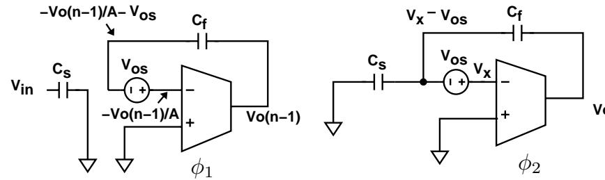
$$V_x = V_o/(-A), \quad (V_o - (V_x - V_{os}))C_f + (0 - (V_x - V_{os}))C_s$$
