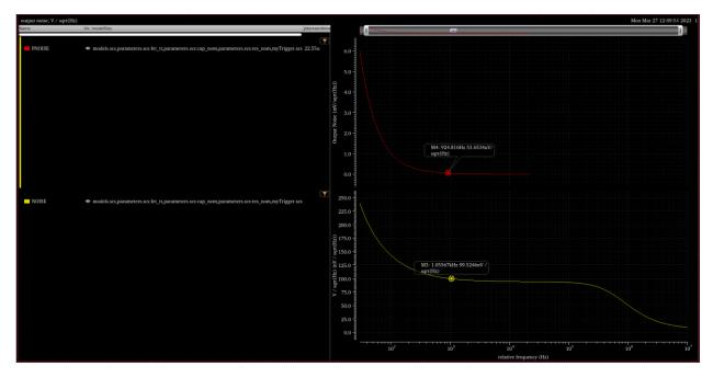
PNOISE (red) vs NOISE (yellow). 53.6uV/rt(Hz) compared to 100nV/rt(Hz) at 1KHz.
