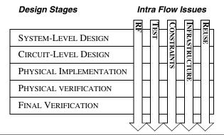
design can be neatly separated into these stages. There are certain design capabilities and tool requirements that span the design process. In many ways these are the more difficult for EDA tool vendors to address as they are not contained wholly within the expertise of a specific design stage, and of necessity require interaction across the designers and design tools at each of these stages. Section 3.0 explores these complex intra flow issues and how they might be addressed.
