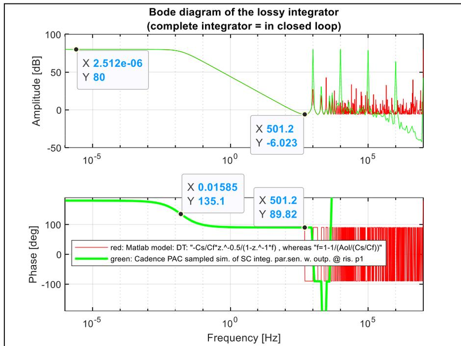
**Figure 4 – Transfer functions of Matlab model (red) and Cadence (green) of the lossy integrator; The Cadence SC circuit is with the data read-out at rising edge of phase “p1”**
