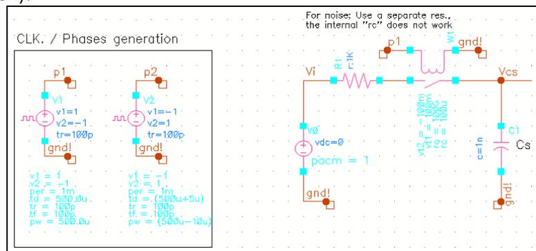
Figure 1 – Test-bench circuit for kT/Cs noise with a Track & Hold (T&H) alone (no subsequent nodes connected where current could flow)
