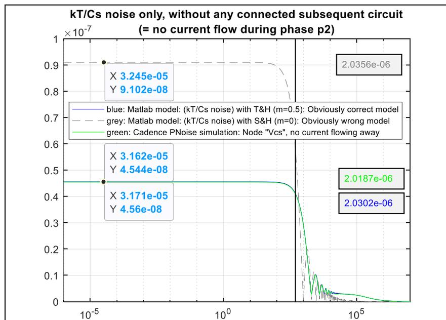
Figure 2 – Matlab model (blue) and Cadence results (green) for kT/Cs noise with a Track & Hold (T&H) alone (no subsequent nodes connected where current could flow)
